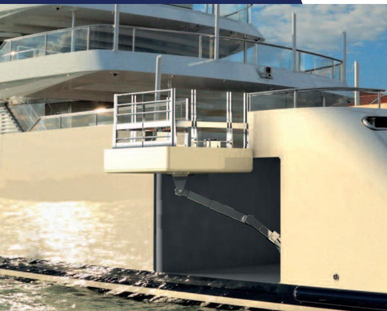
**FLYING CARPET®** is an exclusive, innovative embarkation/disembarkation system for Superyacht. Patented internationally, it is especially intended to carry people but can also be used to facilitate loading and unloading of goods.
